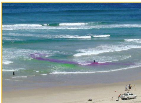
Green and purple dye released in a feeder channel, converging and moving offshore in a rip current. This research was part of a field campaign to measure the pressure-gradient force and the resulting flows within a rip current system off of Moreton Island, Australia.
