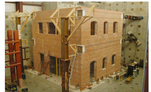
Full-scale testing of unreinforced masonry building.
