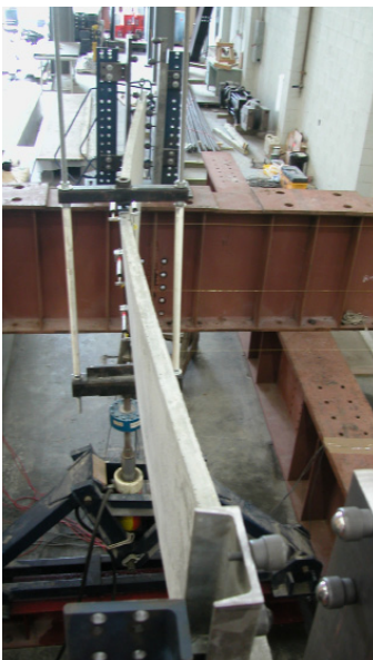
Lateral stability tests of reinforced and prestressed concrete beams.
